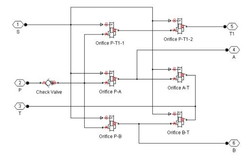
All the orifices in the model are closed (overlapped) in valve neutral position, except orifices  $P_T1_1$  and  $P_T1_2$ . These two orifices should be set open to an extent that allows pump delivery to be discharged at low pressure.
